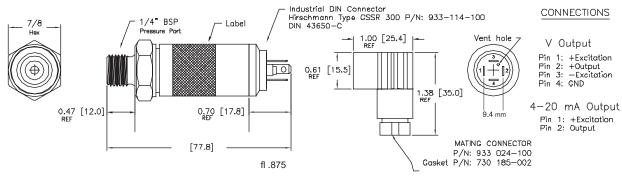
Vent through hole in connector ( under 1000 psi )
