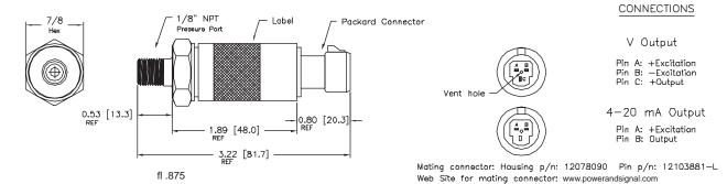
Vent through hole in connector ( under 1000 psi )
