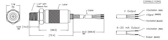
Vent through cable ( under 1000 psi ) Max operating temperature for cable is 100°C.
