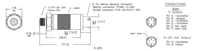
Vent through removed Pin F hole ( under 1000 psi )
