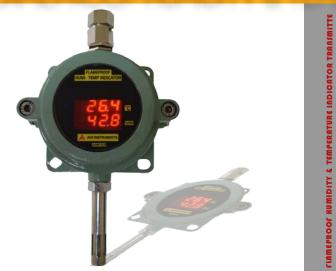
ACE INSTRUMENTS make Flameproof Humidity & Temperature Indicator simultaneously measures %R.H. & Temperature in hazardous area applications. With 2 Analog Outputs of 4-20mA, one each for temperature & humidity along with optional RS485 Modbus communication, the instrument finds immense usage in pharmaceuticals, petrochemicals, bulk, drugs, chemicals, warehouses, pharma clean rooms & other allied applications.
