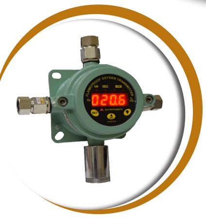
Flameproof Oxygen Monitor Transmitters manufactured by Ace Instruments are high precision microcontroller based gas transmitters housed in flameproof aluminum LM-6 Body certified by CIMFR, Dhanbad for use in Gas Group Areas I, II, IIA & IIB. The 4 digit LED display shows the digital display of oxygen gas concentration in the range of 0.0 to 25.0% Volume.
